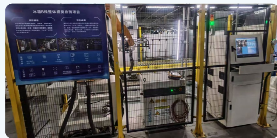
On-site Comprehensive Visual Inspection Project for Refrigerator Production Line B
